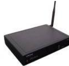
NG Residential gateways: Ethernet Switch, ADSL2/2+, SoftPBX, USB2.0, WiFi a/b/g/e, SD Flash Card UWB, GPON, VDSL, HDTV
